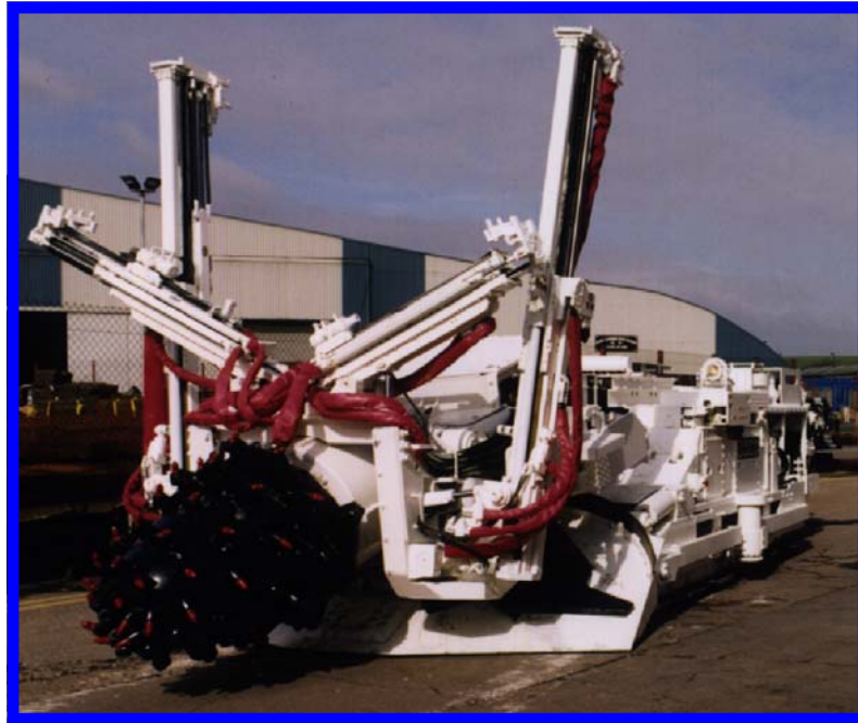
LH 1400 with telescopic boom and 4 drill rigs
